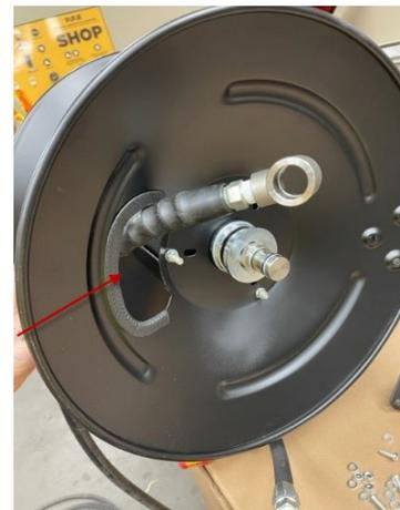
5. RÉINSTALLER LE CORPS PIVOTANT SUR LA TIGE EN S'ASSURANT DE DONNER UNE BELLE COURBURE AU BOYAU
